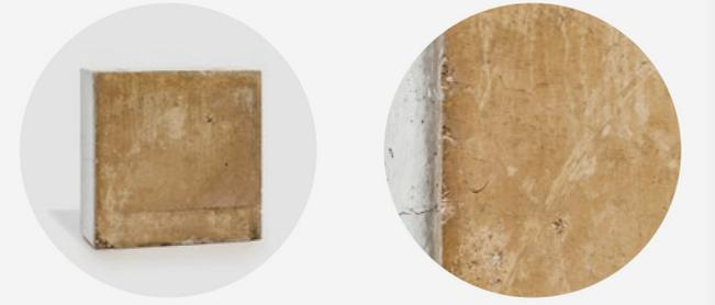
BRE sample with Ignis subjected to European Hydrocarbon Curve showing no spalling
