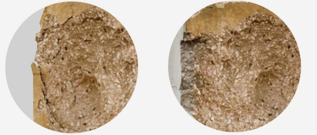
BRE sample without Ignis subjected to European Hydrocarbon Curve showing severe spalling
